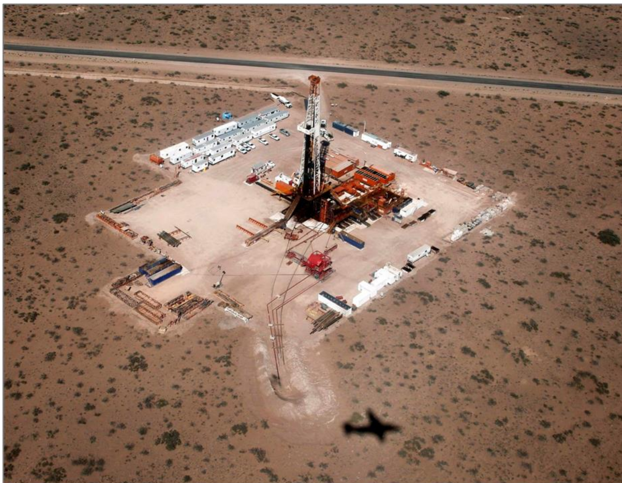
Figure SPM 1.5: Wellpad layout with a drill rig of about 40 m in height within an arid environment in Argentina. (Source: REUTERS, http://www.vcpost.com/articles/5923/20120925/sidewinder-drilling-to-buy-union-drilling-for-139-mln.htm ).
