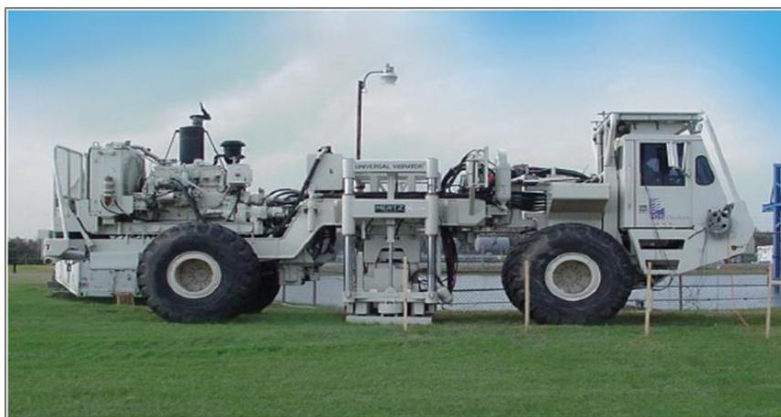
Figure 3-2: Seismic vibration (vibro) truck
