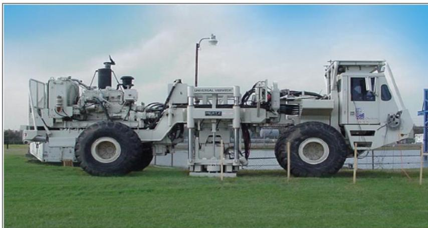
Figure 3-2: Seismic vibration (vibro) truck
