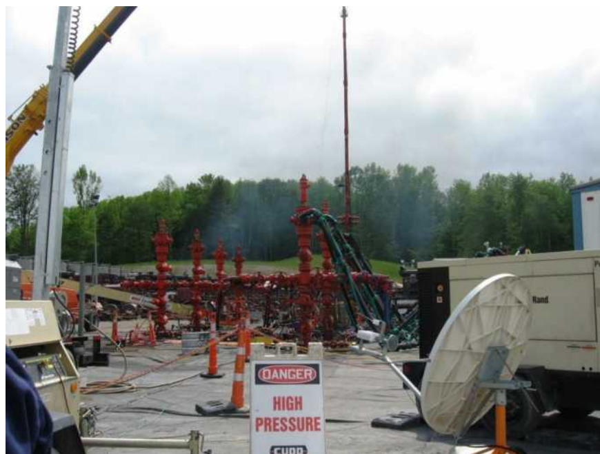
Plate 1.5: Example of an hydraulic fracturing operation underway, involving a series of wellheads (Source: Tom Murphy, Pennsylvania State University, USA).
