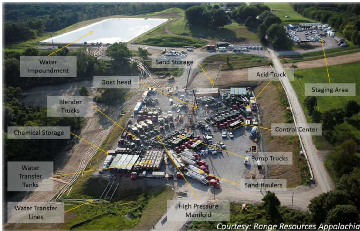
Plate 1.4: Example of an hydraulic fracturing process underway in Appalachia, with the main equipment and facilities involved indicated. (Source: Range Resources Corporation).
