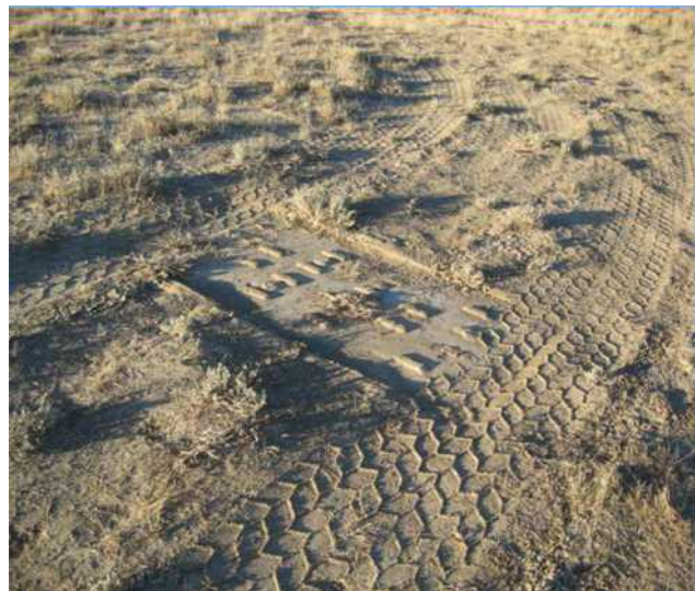
Plate 1.2: Ground impression left by the vibrator pad of a vibroseis truck (Source: Shell).
