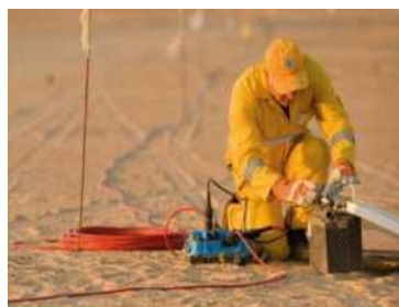
Personnel setting up a seismic data collection system, which includes a small recording box, a battery, and an array of geophones). Fibre optic cables laid out in a grid pattern over the survey area transmit the signal from the recording box to the recording truck (Source: Shell)
