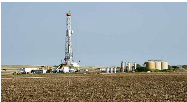
Figure 14.4: Wellpad with drilling rig (earthtimes.org)
