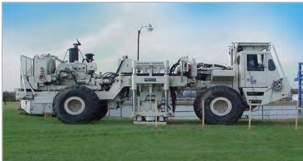
Figure 1.20: Seismic vibration (vibroseis) truck ( Source: Shell ).
