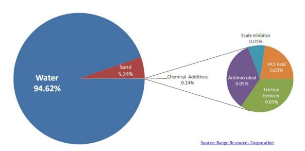
Figure 3–5: Example of the relative composition (% contribution to total volume) of compounds comprising a typical batch of hydraulic fracturing fluid (Burns et al., 2016)
