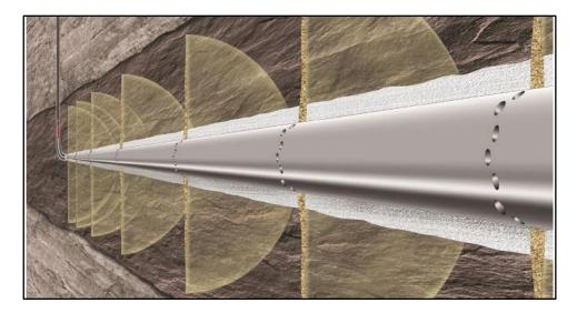
Figure 3–4: Schematic illustration of a horizontal wellbore with perforations through which fluid is transmitted into the surrounding shale (Burns et al., 2016).
