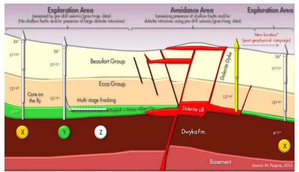
\*Original proposed well (in yellow) will be moved within the same farm if the geophysical campaign revealed the presence of dolerite sill
