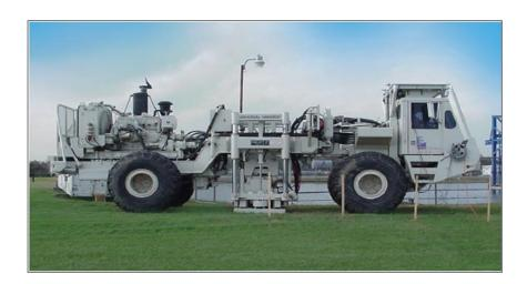
Figure 3–2: Seismic vibration (vibroseis) truck
